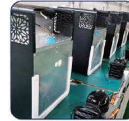
Vacuum pumping and refrigerant filling
